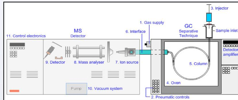
Figure 4. A diagram of the Gas Chromatography-Mass Spectrometry apparatus (CHROMacademy).
