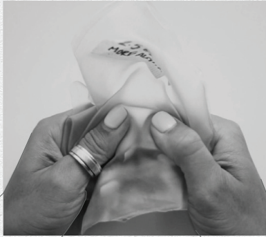
Figure 5: Calcium Alginate biopolymer sheet: flexible substrate for nanowires
