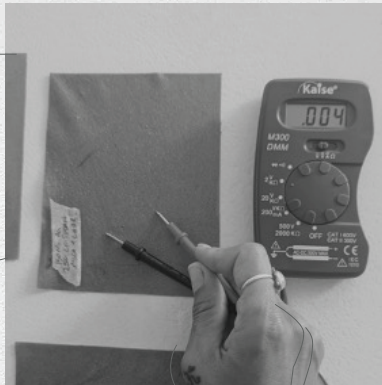
Figure 6: Calcium Alginate embedded with activated charcoal and graphite to test conductivity of composite material.
