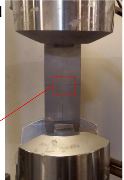
Fatigue test for crack generation
