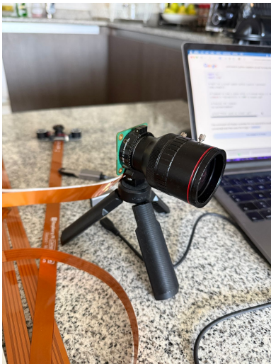
FIGURE 5. Optical camera chosen (A) in small tripod on desk test. In B a picture taken on desk, controlled by Raspberry Pi5, using python algorithms. In C a close up of the capabilities of Raspberry Pi5, showing several (4) USB ports, video displays (two ports), one HDMI and ethernet connector.
