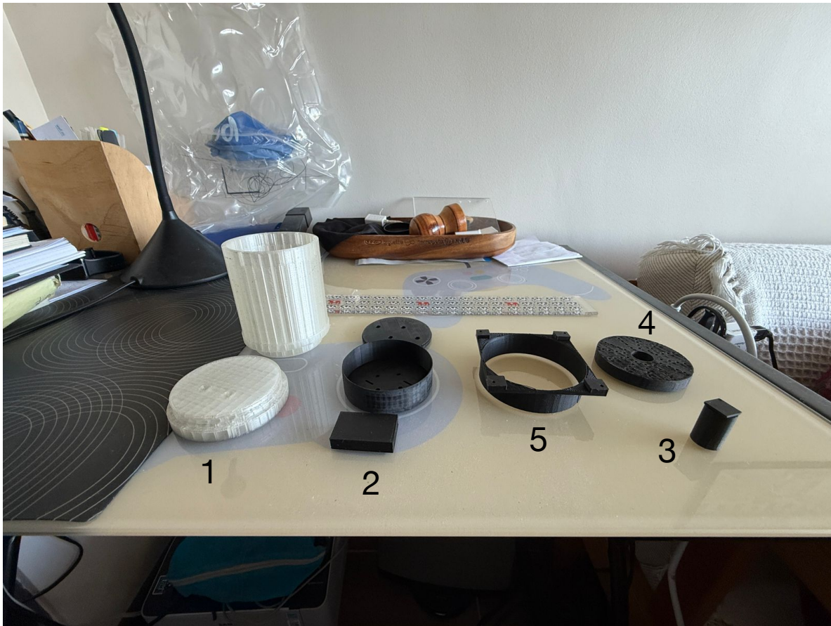
Figura 2. Model in 3D at scale of the components to hold the electronics and optical elements of the HySPI. In white (1), The whole Chamber build in bullet proof acrylic and the cover with o-ring to provide a water tight environment. The cover will bear 2 connections points for tethering to surface the HySPI. In black, number 2, 3 and 4, are internal sections that will be held inside the chamber. Number 2, is a sub chamber that will hold the controlling unit (raspberry Pi5 = small box) that will be inside the round box and covered. Bottom and cover wear connectors passages (round holes and square ones) to allow connection within the chamber elements (LED and Camera CMOS). Number 3 is mock volume of the CMOS camera, lens and control; this camera will be held in position vertical in the central hole of number 4. This latter will hold the LEDs that will be evenly distributed to achieve a fair illumination inside the MSU.
